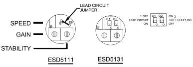
Switch 1 controls the "Lead Circuit" found in the ESD5111. The normal position is "ON." Move the switch to the "OFF" position if there is fast instability in the system.
